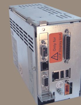
PC unit with CTM card (in switch cabinet), visualization, e.g. via TCU of the Siemens SL
