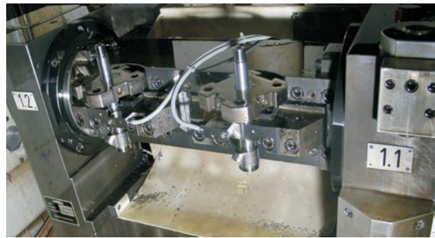
Fig. 2: Acoustic emission sensors on each clamping point in order to receive an "optimum" signal.
